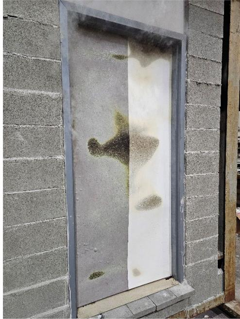
**Figure 6:** The unexposed side 7 min into test
