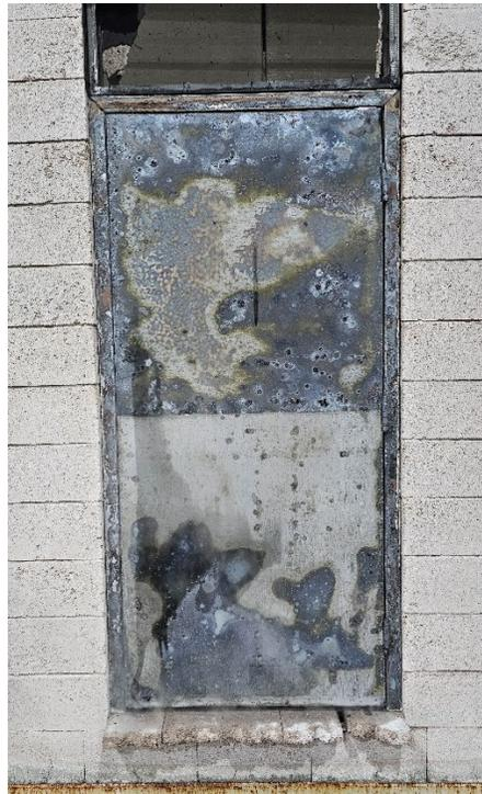
**Figure 9:** The exposed side after the hose stream test.
