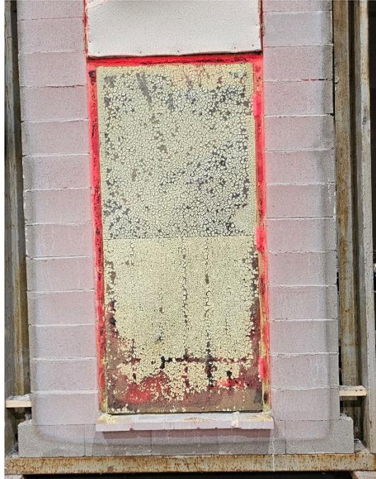
**Figure 8:** The exposed face at the end of the fire test.
