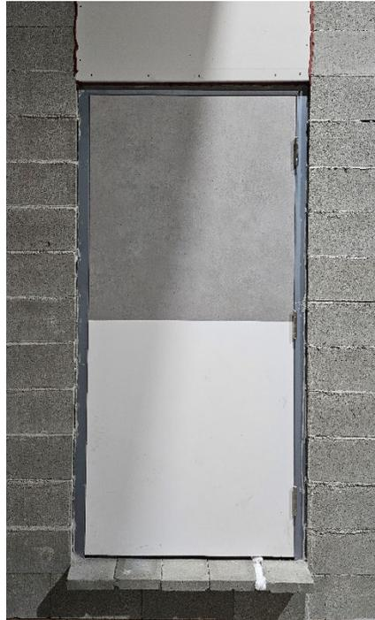
**Figure 4:** The exposed side prior to the fire test.
