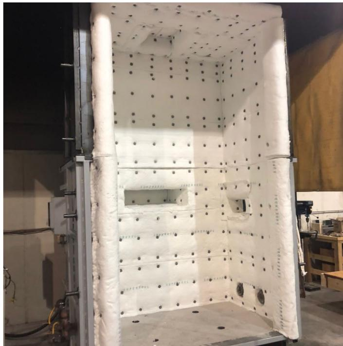
**Figure 1: Test Furnace**
